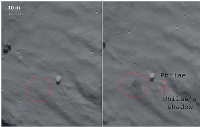
fig. 4. On the left, photograph of Agilkia surface before landing; the red circle indicates the area where Philae subsequently impacted; on the right, photograph taken 1.5 minutes after touchdown; one can see Philae just bounced, casting its shadow on the ground; inside the left circle, the cloud of debris raised by the collision is visible. Credits: ESA/Rosetta/NAVCAM, The Telegraph; edited by the author.
