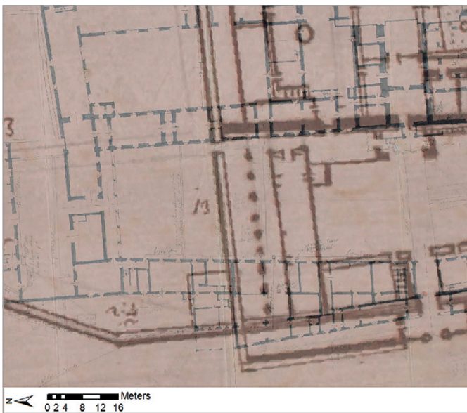
fig. 8. The overlay of the 1688 and 20 th -century maps, achieved in a GIS environment, enlightens the transformations of the Cortile d'Onore happened in the late 18 th century.
