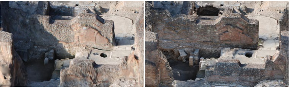
Figure 3: Rome, NE Palatine slopes. (a) Portion of the 3D model recently reprocessed with the CNR photographic archive, using multi-image photogrammetry; (b) the same portion of 3D model integrated by processing dataset acquired in the last topographic and photogrammetric survey.
